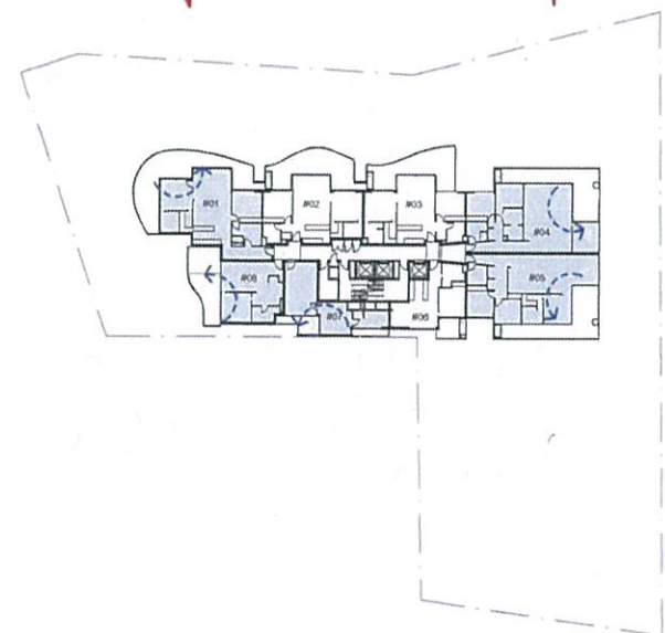
6 NATURAL CROSS VENTILATION - L5 - L10 (TYPICAL) 1:500
